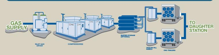
**DAUGHTER SYSTEMS** are installed where a CNG fill station utilizes mobile CNG storage as the fuel source for the station.
