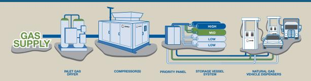
**TIME FILL SYSTEMS** are a cost effective fueling option that allow vehicles to conveniently refuel overnight or when the vehicles are not in use.
