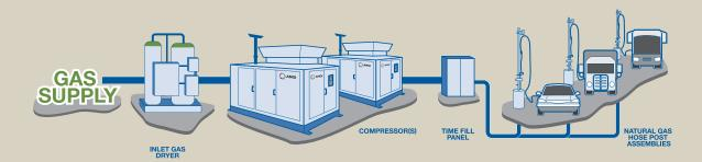
**COMBINATION SYSTEMS** feature both a fast fill and time fill system allowing high utilization of the compression capacity both day and night.
